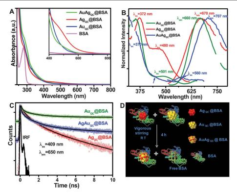
**Fig. 2** (A) UV–Vis spectra of BSA,  $Au_{QC}$ ,  $Ag_{QC}$ , and  $AuAg_{QC}$ @BSA. (B) PL spectra of  $Au_{QC}$  (green line),  $Ag_{QC}$  (red line), and  $AuAg_{QC}$  (blue line) @BSA. Emission spectra were collected for all the three clusters by exciting them at 370 nm. (C) Picosecond-resolved fluorescence transients of  $Au_{QC}$ (green),  $Ag_{QC}$  (red),  $AuAg_{QC}$  (blue) @BSA. (D) Schematic of the synthesis of AuAg@BSA alloy clusters through QC–QC interaction.
