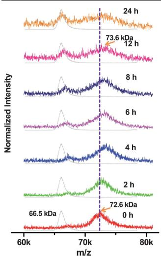
Fig. 3 Time-dependent MALDI MS data of AuAg<sub>QC</sub>@BSA show the emergence of the free protein and also the shifting of the cluster-containing protein peak from m/z 72 600 (0 h) towards m/z 73 600 (12 h) as a function of time.
