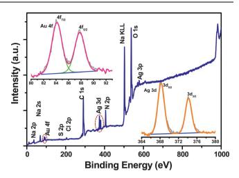
**Fig. 4** XPS survey spectrum of  $AuAg_{QC}@BSA$  showing the presence of metallic Ag and Au (dotted pink circles). Inset: expanded and fitted spectral regions of Au 4f (magenta line) and Ag 3d (orange line).
