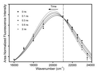
Fig. 5. Time-resolved area-normalized emission spectra (TRANES) of the dansyl probe in micellar environment at five delay times from t = 0 ns. Note the isoemissive point at 21066 cm<sup>-1</sup> (see text).
