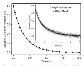
Fig. 4. The solvation correlation function, C(t) of the micellar environment probed with the dansyl chromophore. Inset shows time-resolved anisotropy, r(t) decay of the dansyl probe in the micellar environment.
