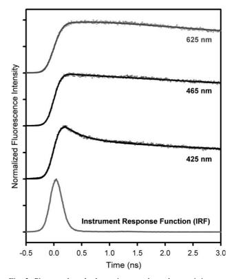
Fig. 2. Picosecond-resolved transients at three characteristic wavelengths of the dansyl probe in micelle. Transients are normalized for comparison.
