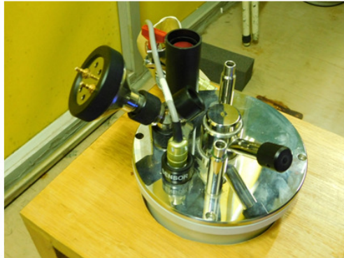
Cryostat for low temperature Photoconductivity measurements down to 77K
