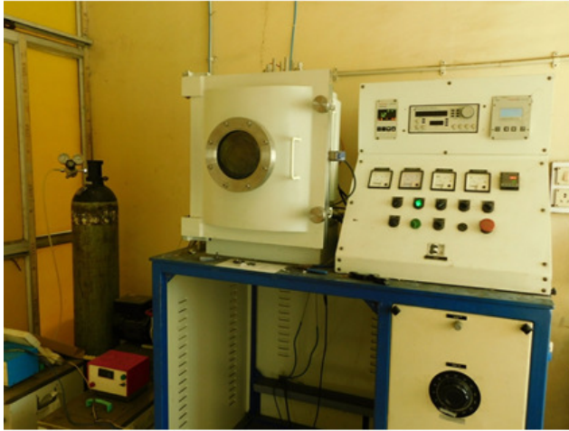
Thermal evaporation unit for metal deposition
