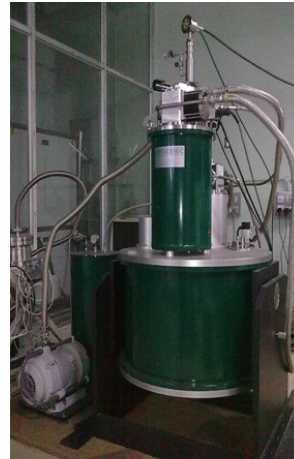
1.5K, 10T GM cycle based low temperature system for transport, magnetic, Hall and dielectric measurements.
