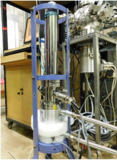
Cryostat with UHV set-up along with electronics
