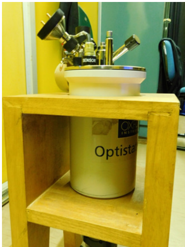
Cryostat for low temperature Photoconductivity measurements down to 77K
