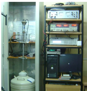
Low frequency noise Measurement and with variable temperature facility down to 77K with magnetic field of 0.4T
