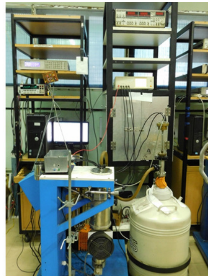
Resistivity & impedance measurement set-up down to 77K
